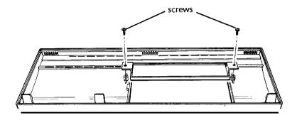
Set the front panel, slot cover, and screws aside.
